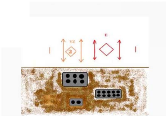
2 Single Double ended Arrows With a Diamond in between. This mark will be on any Multiple Duct Structure
